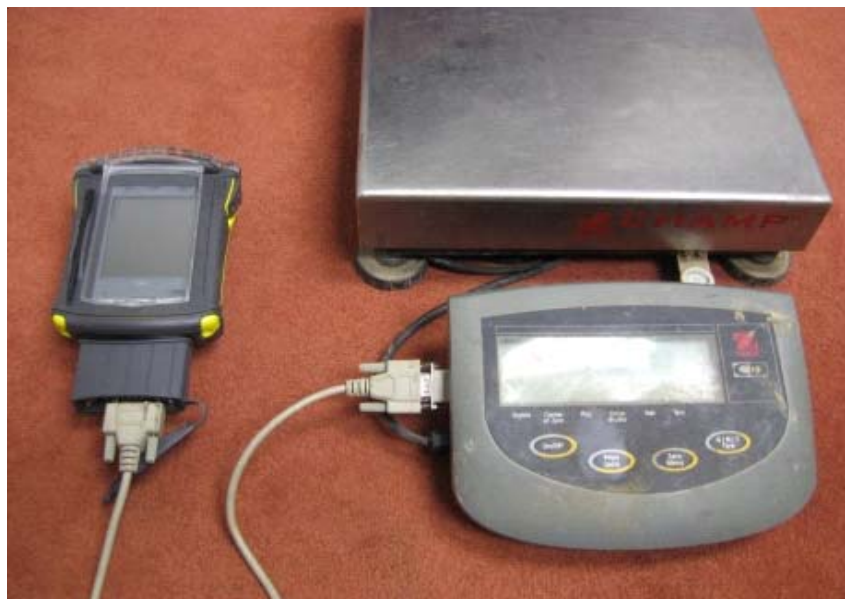
Figure 15. Equipment used to efficiently assess the size distribution of large fish samples.
