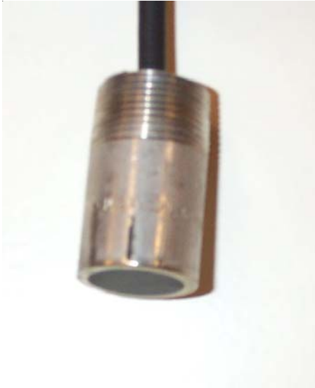
Figure 7. 460 kHz transducer designed for the individual catfish sizing system.
